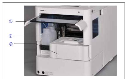
Fig. 16 Autosampler with additional container for transporting samples
