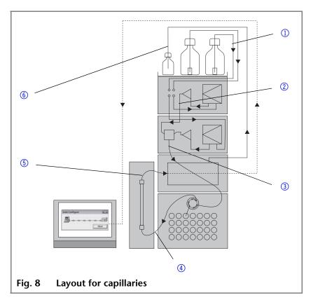
Details on stainless-steel capillaries in HPG system
