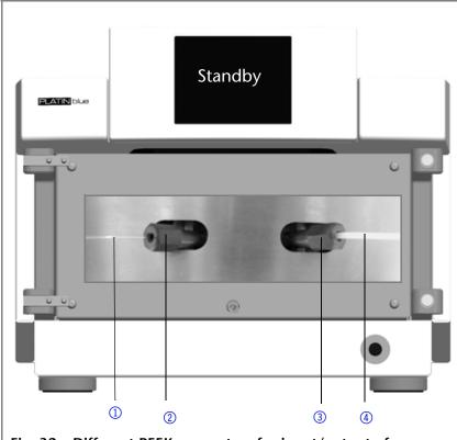
Fig. 32 Different PEEK connectors for input/output of measuring cell on PDA-1
