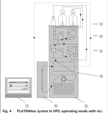
Fig. 4 PLATINblue system in HPG operating mode with recommended installation of capillaries
