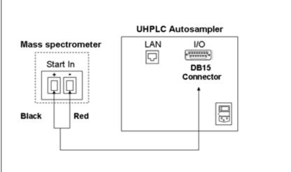
Fig. 34 Schematic display of connections for mass spectrometer and autosampler
