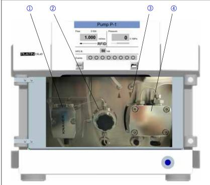
Fig. 14 HPG pump with pressure sensor, mixing chamber and steel capillaries from mixing chamber to autosampler
