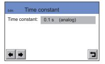
Fig. 64 Selecting time constants for detectors
