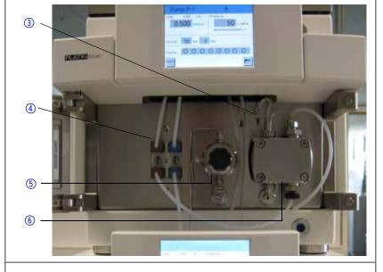
HPG pump P-1 with HPG mixing chamber ①, pressure sensor, venting valve and pump head
