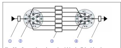
Fig. 22 Connection schematic within the T-1 with valves
