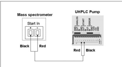
Fig. 35 Schematic display of connections for mass spectrometer and high-pressure pump
