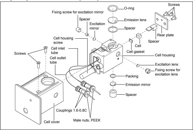
Component parts of the flow cell unit (RF-20A)
