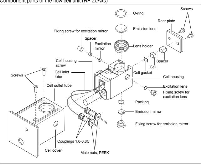
Component parts of the flow cell unit (RF-20Axs)
