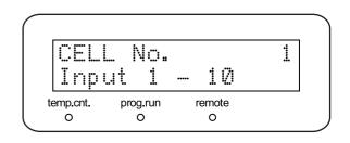
Upon entering the cell number set for this instrument, the instrument operates based on the wavelength calibration data that corresponds to the set cell.
