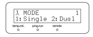
5 Enter 2 and press enter. This sets the measurement mode to dual wavelength.
