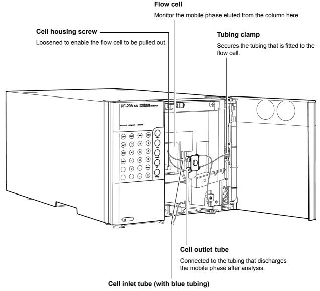
Connect the tubing from the column here.
