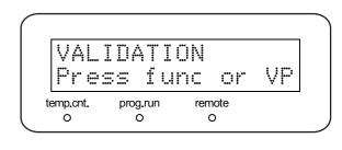
2 Repeatedly press **func** until [LEAK SENSOR TEST] appears.
