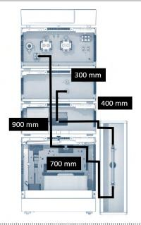
System 4: AZURA® analytical with manual injection, DAD and RI detector
