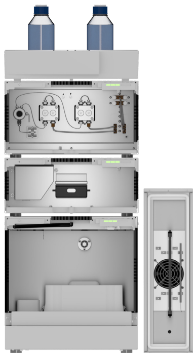
Fig. 12 System setup of analytical HPLC system; left from top to bottom: eluent tray with bottles, pump, detector, autosampler; right: column thermostat with column.
