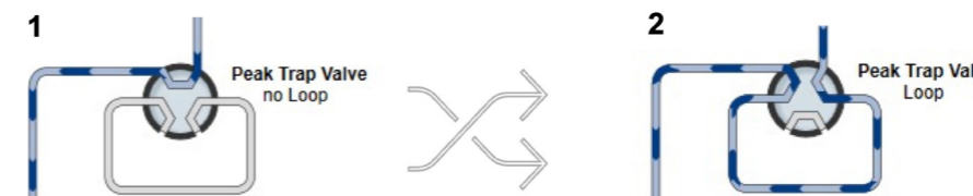
Fig. 4 Two flow paths for the peak trap valve. 1) Flow bypasses the peak trap. 2) Flow passes through the peak trap. Peak trap loop or column.
