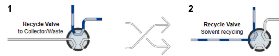
Fig. 5 Two flow paths for the recycle valve. 1) Flow goes to the collector/waste. 2) Flow is being recycled.
