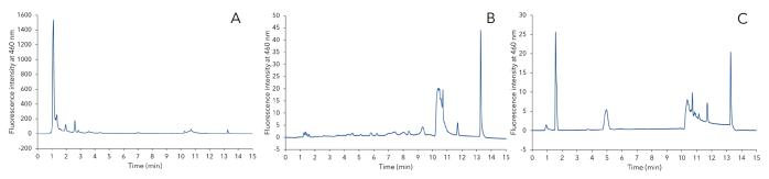
Fig. 2 Three different samples during extraction process. After the extraction with MeOH/H<sub>2</sub>O (A), before SPE (B) and after the SPE extraction (C).
