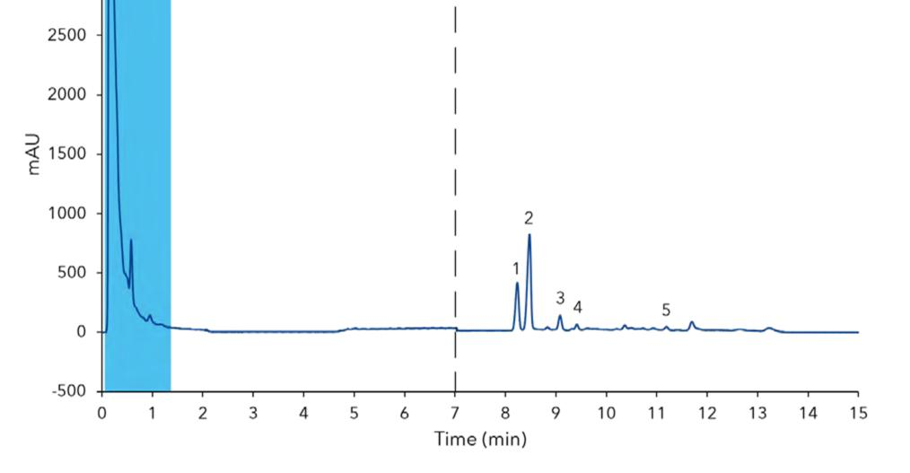
**Fig. 1** Measurement of washing process; blue area: matrix; 1) rebaudioside A, 2) stevioside, 3) rebaudioside C, 4) dulcoside A, 5) steviolbioside; 20 μL injection of Stevia extract; 0-7 min) measuring of SPE Washing Process, 7-15 min) measuring of HPLC
